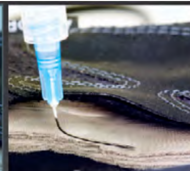
25 gauge needle failure
