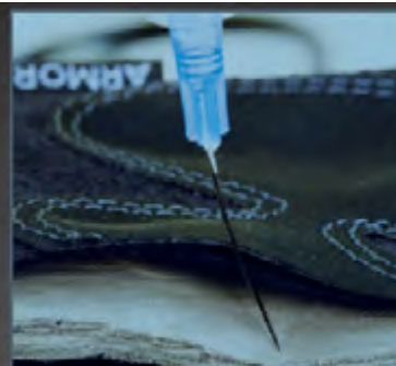
25 gauge needle buckling
